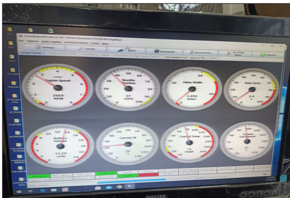
Figure 5. Tuner Studio software for the air assist injector
